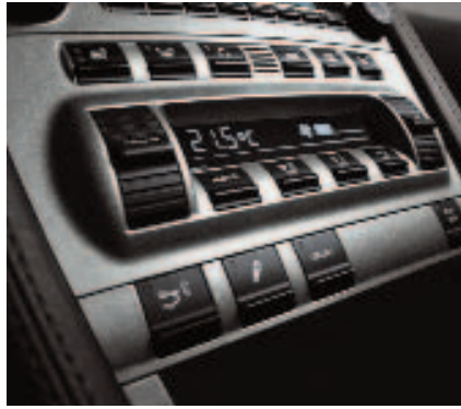
Fig. 64: Control panel for the air conditioning system
