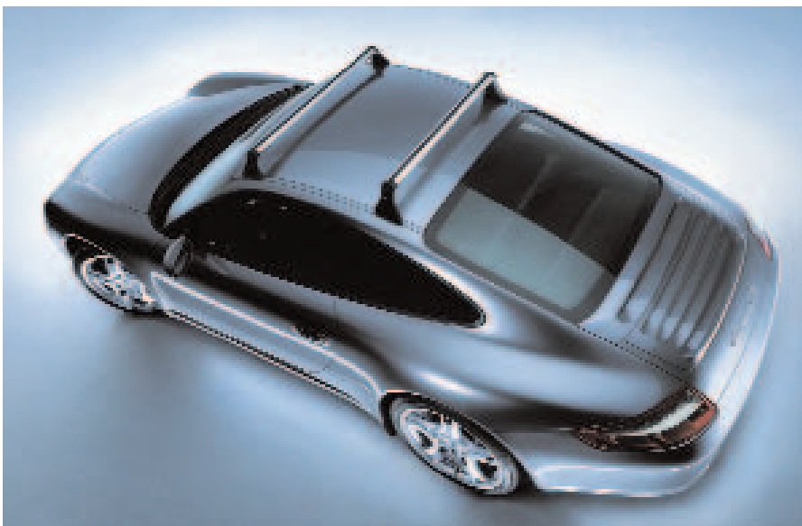
Fig. 49: Roof transport system
