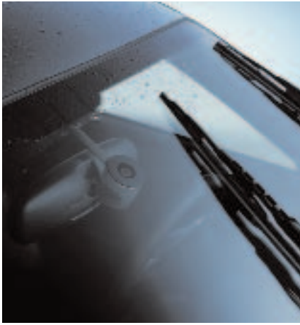
Fig. 71: Interior mirror with rain sensor
